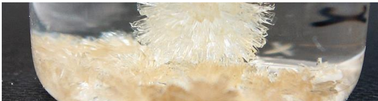
Crystals of GUT-2. For the choice of the name of a metal-organic framework, in any cases the acronym of the research institution is chosen followed by a consecutive number.
