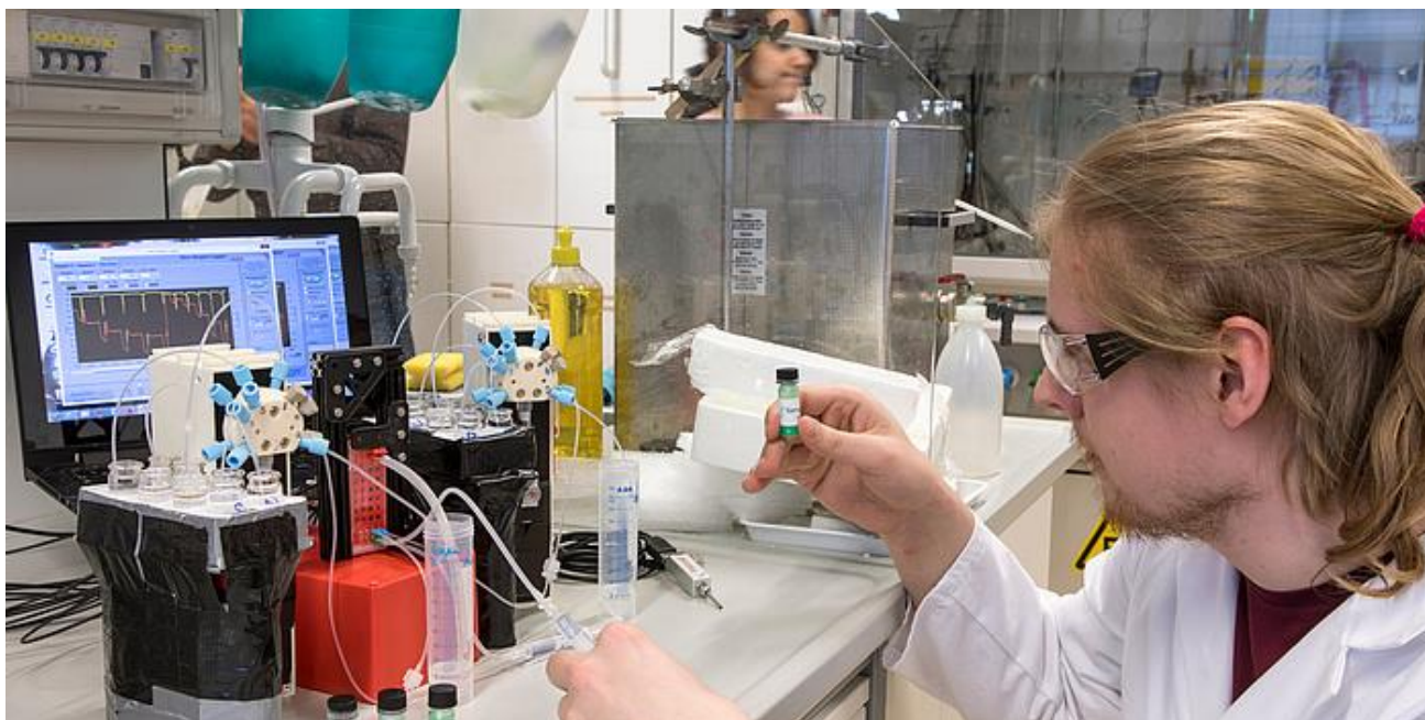
Typical set-up of microfluidic reactors. Reagents and fluids are injected into the reactor using syringe pumps. The reaction can be controlled in real-time with the integrated sensors.
