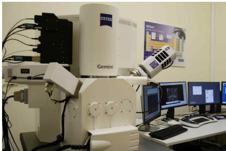
Fig. 1: The scanning electron microscope Zeiss Sigma 300 VP, with the Raman microscope from WITec (left) and the EDXS detector from Oxford (right).
