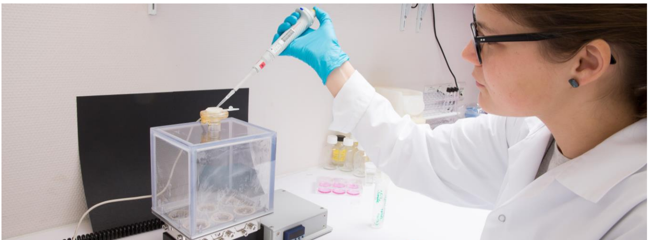
Exposure of cells to a solution using the VitroCell Cloud chamber. © LIST
