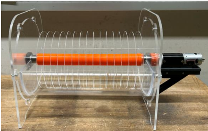
5-L rotating disc reactor for bacterial cellulose production.
