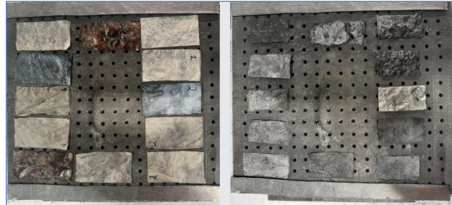
Functionalised bacterial cellulose before/after carbonisation procedure.
