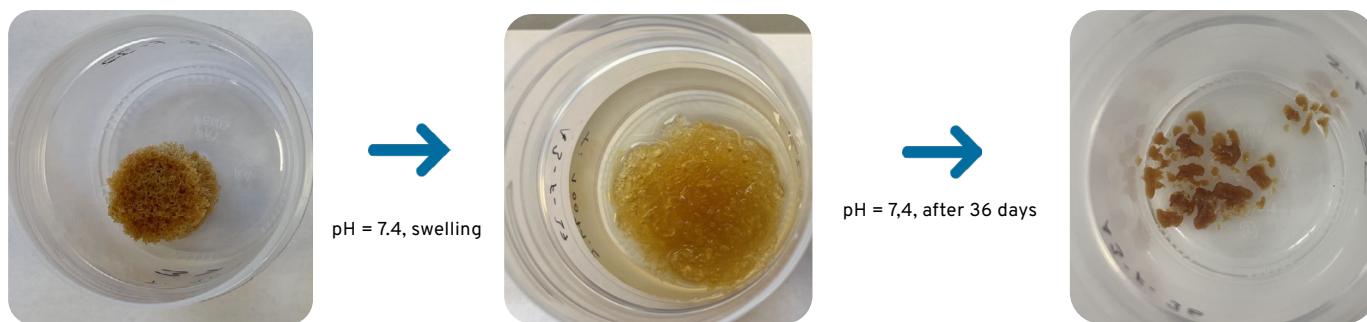
Swelling and degradation of an APtA-PU foam in a buffered solution (PBS) at pH 7. Left – dry foam; middle – foam after 7 days in the buffered solution; right: foam after 36 days (dried).
